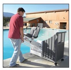
Push lift to deck side, set brakes, slide into place and it's ready to use.
